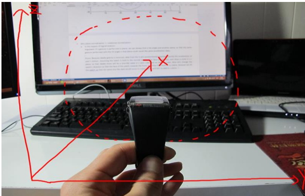
Figure 4. A circle is drawn (the dotted line) in the yz plane when the watch is tilted up.
